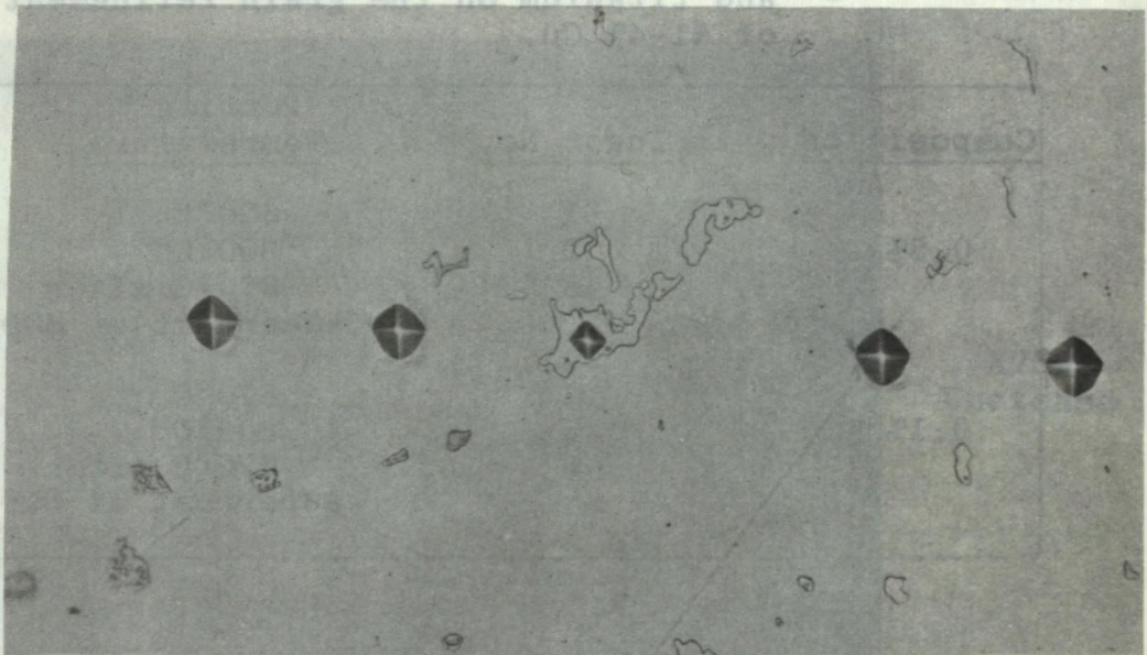
Figure 13. Microhardness indentations on the same alloy as Figure 12. The average value for the nickel matrix was 96 DPH, while the secondary constituent gave values from 220 DPH (as here) to 500 DPH.
