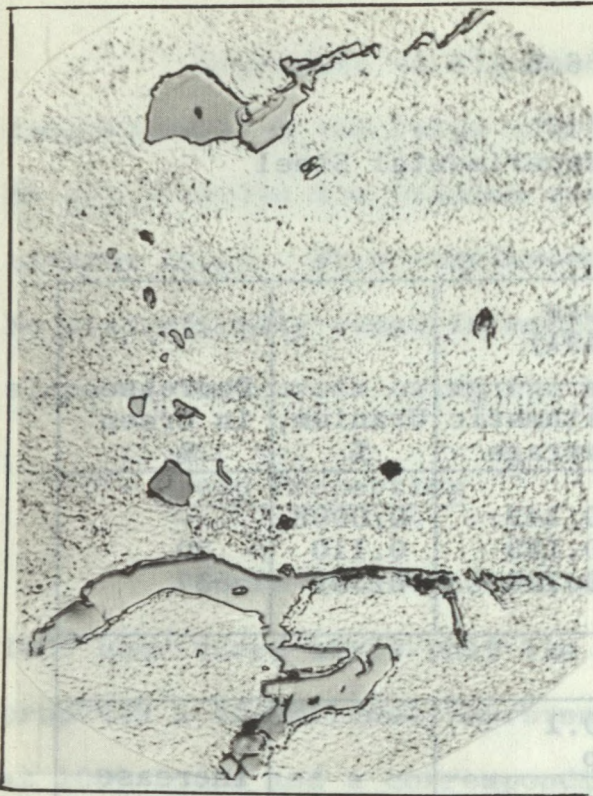
Figure 6.4 - Heat 4358, Specimen IC, As-Cast, Furnace-Cooled From 1040°C (1900°F). (2.11% U). Etched in Villela's Reagent. X750
