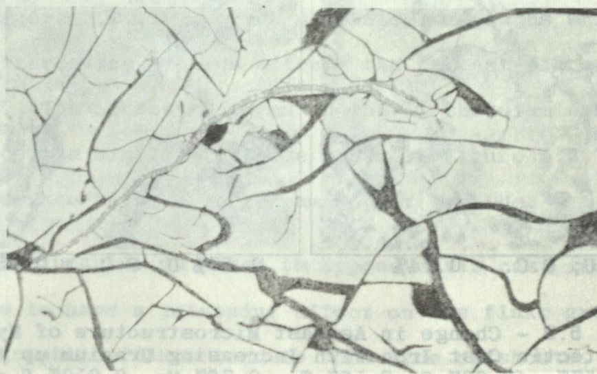
Figure 5.4. - Photomicrograph of High-sulphur Hypereutectic Cast Iron Containing 1.20% Uranium, Showing Fine, Film-type Inclusion and Very Fine Graphite Flakes. As-polished. X500
