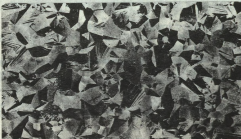
Figure 6. Surface appearance of high-lead coating prepared under the same conditions as for sample in Figure 5 except for presence of 0.15% Sn and 1.0% Pb. X1.
