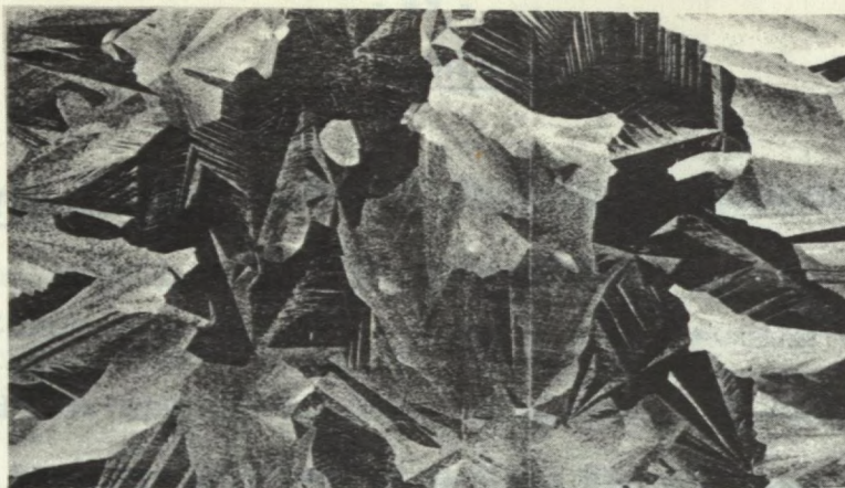
(a) 80 sec immersion at 465°C (869°F). 0.60% Sn, 0.60% Cd, 0.15% Cu, 0.04% Sb, 0.05% Al, 0.5% Pb, 0.03% Fe.
