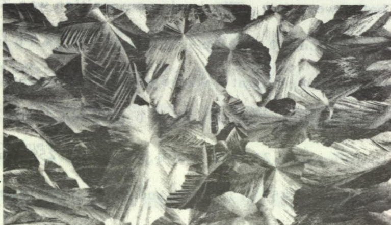
(b) 80 sec immersion at 465°C (869°F). 0.60% Sn, 0.15% Cd, 0.60% Cu, 0.04% Sb, 0.05% Al, 0.5% Pb, 0.03% Fe.
