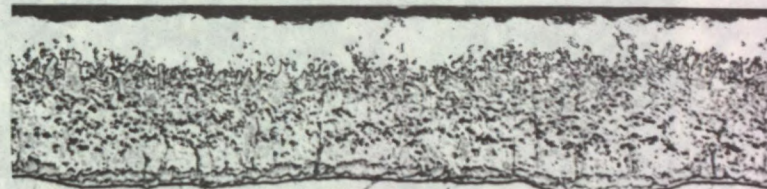
(a) 80 sec immersion at 445°C (833°F). 0.15% Sn, 0.15% Cd, 0.15% Cu, 0.04% Sb, 0.05% Al, 0.5% Pb, 0.03% Fe.
