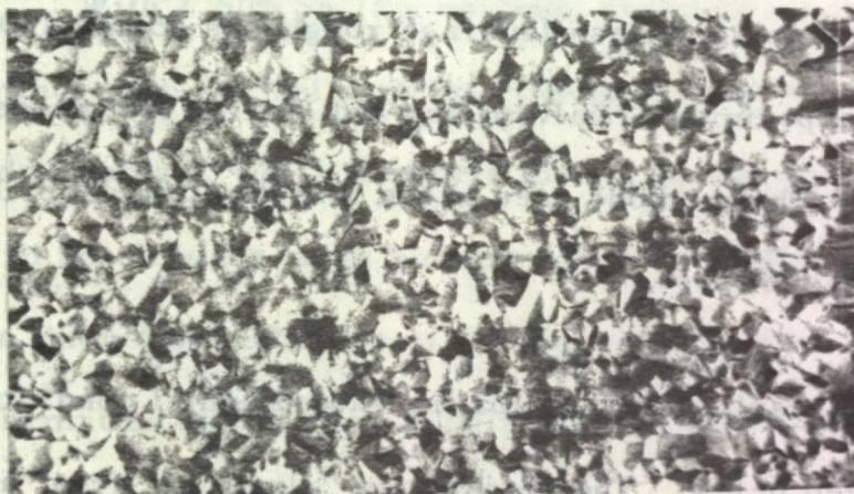
(c) 20 sec immersion at 445°C (833°F). 0.15% Sn, 0.60% Cd, 0.60% Cu, 0.04% Sb, 0.05% Al, 0.5% Pb, 0.03% Fe.
