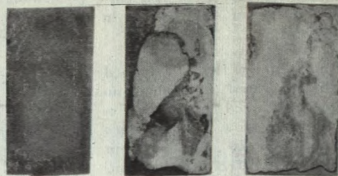
Figure 5.—Under surfaces of horizontal parts of L-shaped panels after cleaning; same specimens as shown in Figure 4. Light areas were the most deeply corroded.
