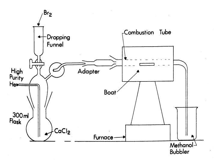
Figure 1. Bromination apparatus.
