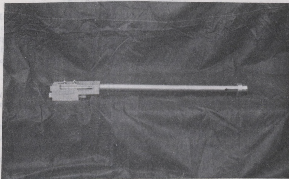
Figure 6. Photograph of gun used for shear wave generation.
