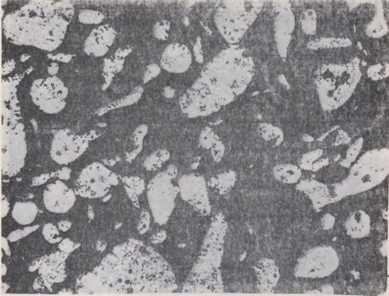
Figure 1 - Al-25% Si alloy powder, -100 mesh.
