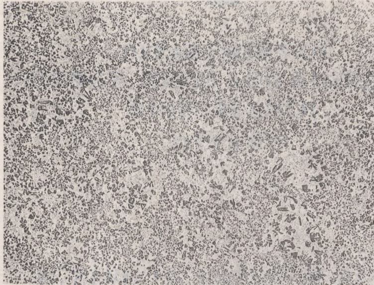
Figure 5 - Hot compacted Al-35% Si alloy powder.
