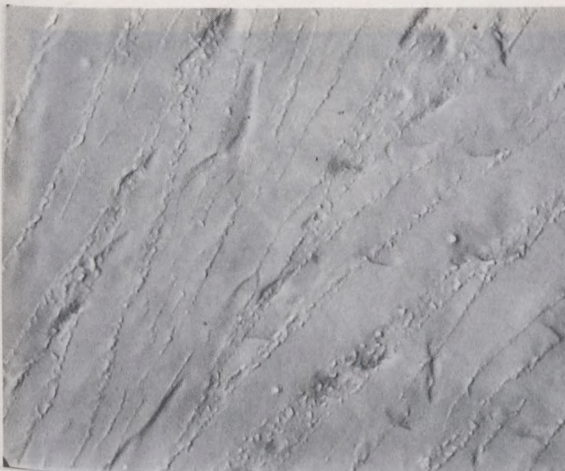
Figure 5 - Zr-0.5% Cu-0.5% Mo. H.T. 1000°C (1830°F), W.Q.; aged 24 hr at 500°C (930°F); as-polished.
