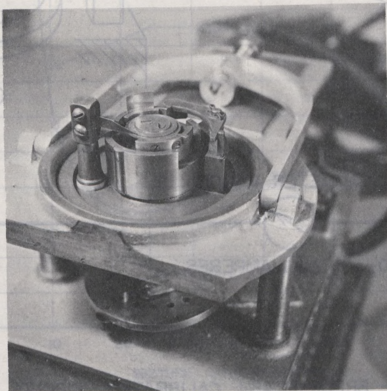
Figure 1. Top - Break-Flash Assembly Bottom - Close-up of Moving and Stationary Electrodes
