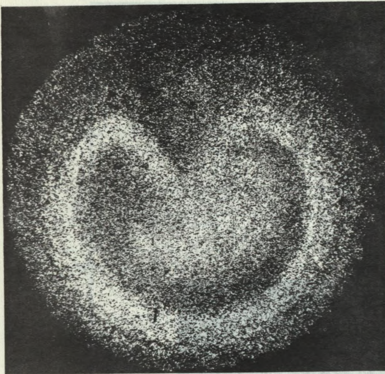
Figure 5. Cross-section through reduced part of ZK61 test bar, etched in 2:2.5:95.5 HF:HNO 3 :H 2 O. Shows light band some distance from the edge.
