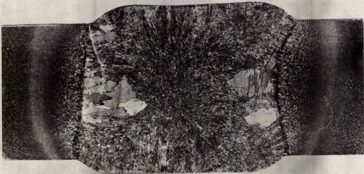
Figure 17. From weld specimen MR16. Electroslag process, Linde MC-70 electrode, Linde 124 flux, vertical-up position.
