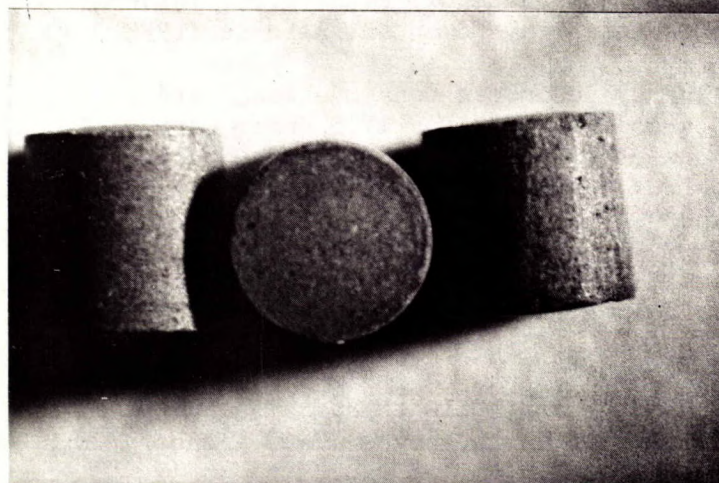
Catalyst used with Leduc pitch. (regenerated 3 times)
