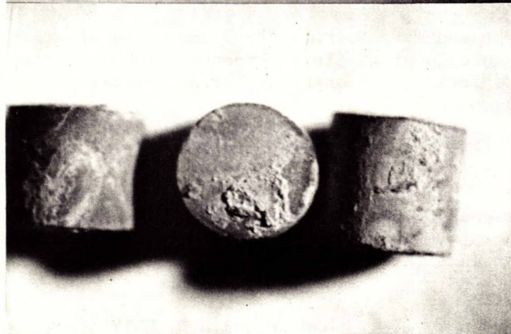
Catalyst used with Athabasca bitumen. (regenerated 3 times)
