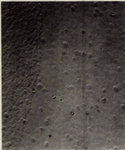
(a) (100) surface with tramp grain on left side.
