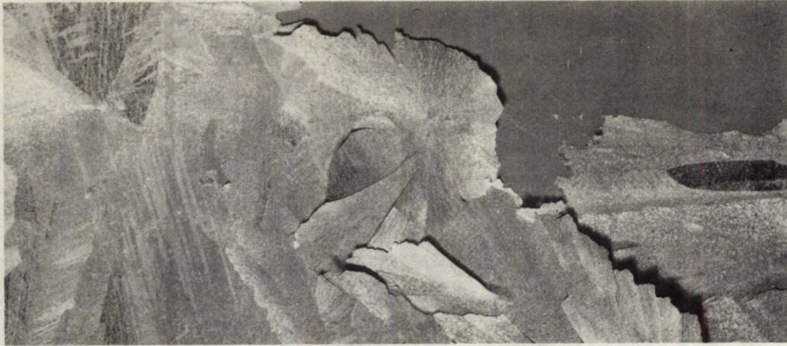
Figure 2. Peeling and break-up of coating (0.5% Pb, 0.10% Al, 1.20% Sn, 0.30% Cd, 0.30% Cu, 0.03% Fe) after heating for 16 hours at 335°C (635°F). X3
