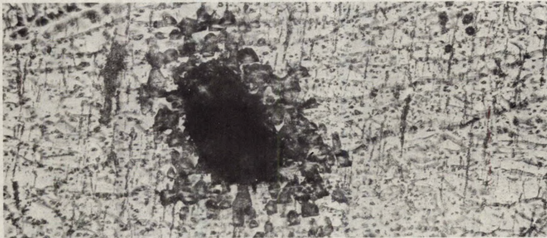
(a) Surface pitting around local iron-zinc alloy growth. X300
