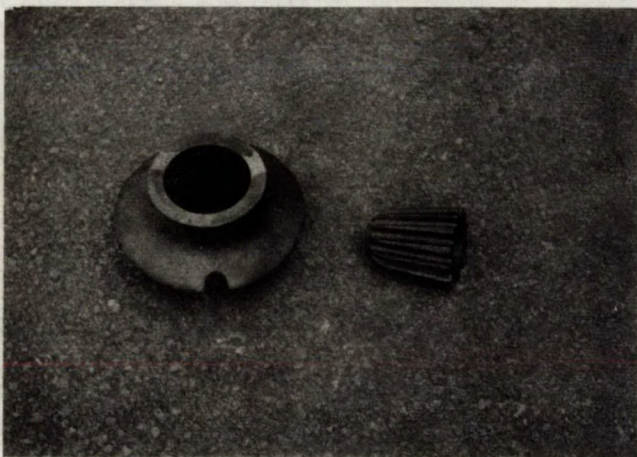
39. Cone and Wedge to Lock Cable.
