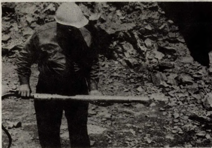
5. Borehole Television Camera.
