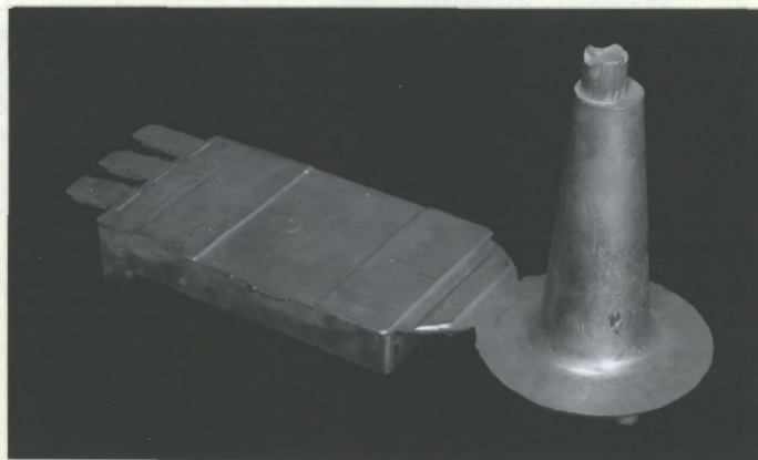
ASTM test casting, showing cover surface .
