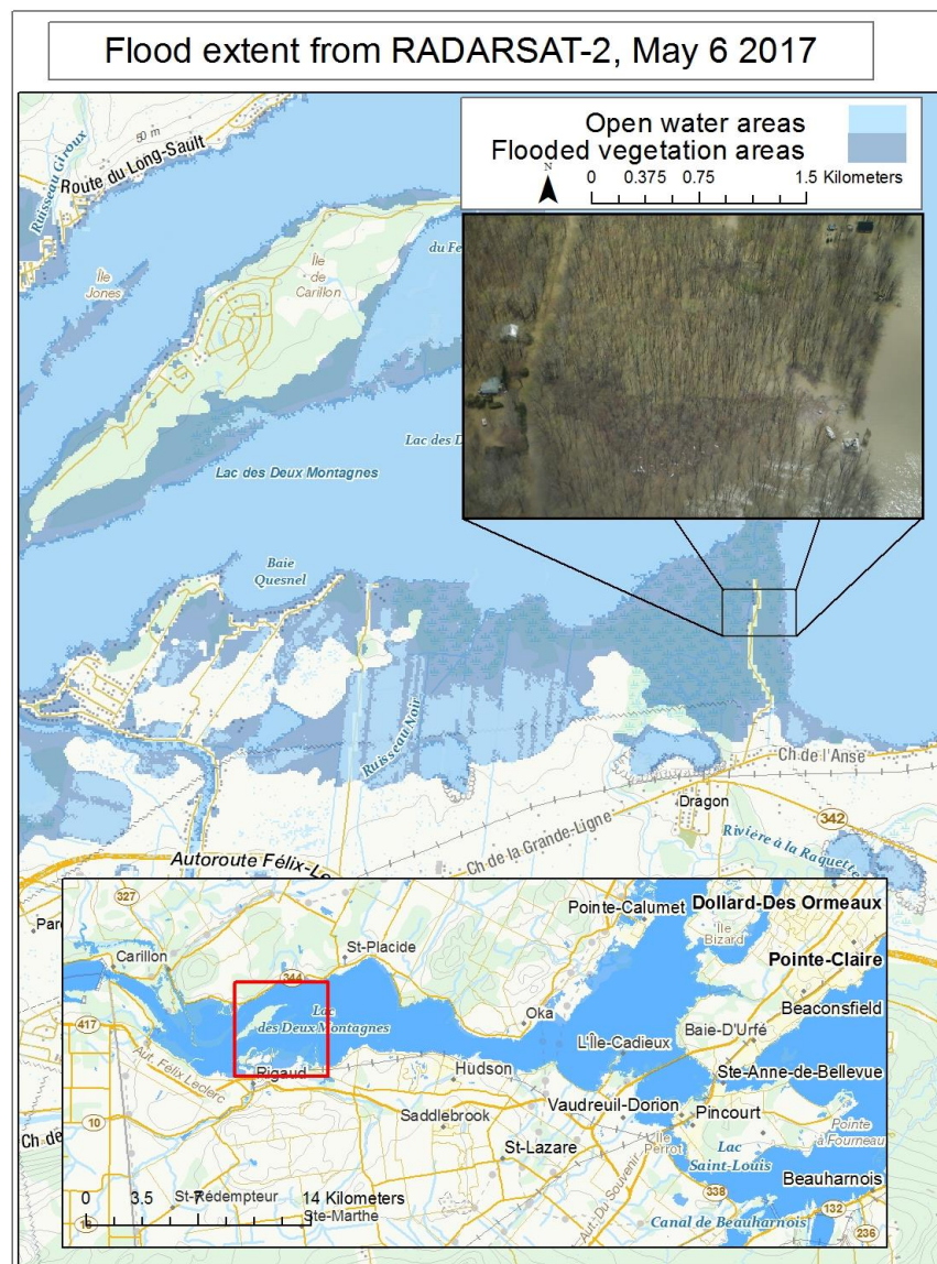
Figure 2. Open water and flooded vegetation mapped from RADARSAT-2 near Rigaud, Quebec, confirmed by oblique airphotos
