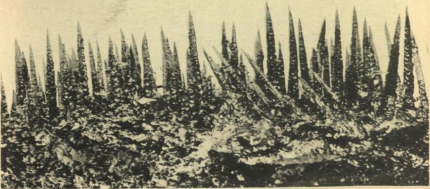
Fused alumina crystals. (Magnified, 4 diam.)
