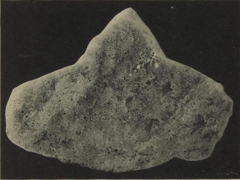
A. Special fused alumina made from amorphous alumina.
