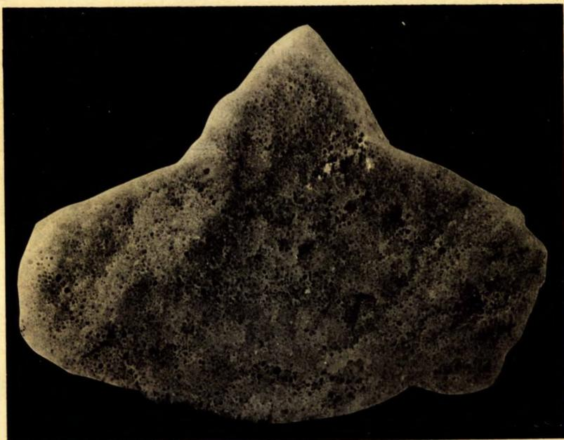
A. Special fused alumina made from amorphous alumina.
