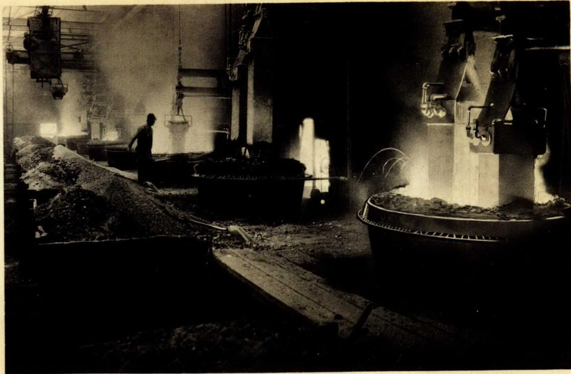
Fused alumina furnace (Hutchins type) in operation.
