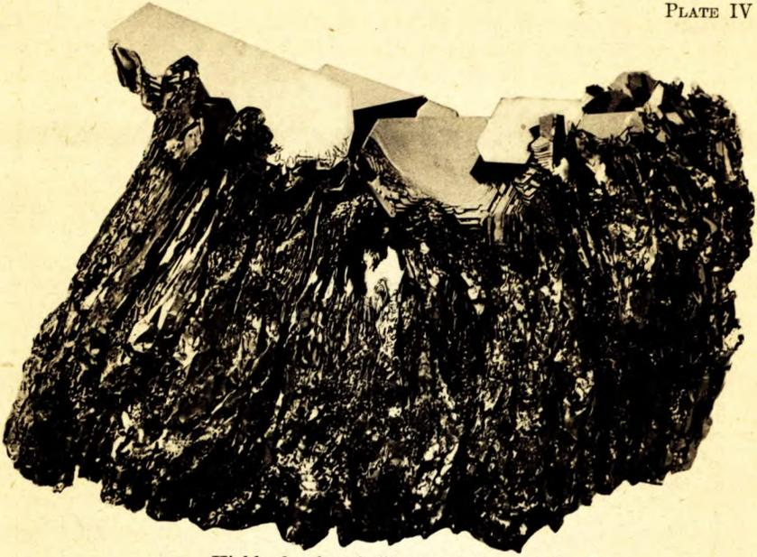
Highly developed silicon carbide crystals
