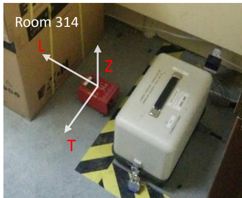
Figure 2. Locations and photographs of the west wing sites. Floor plans adapted from Glazer (2016). Red stars indicate the locations of the Tromino (red box) and the permanent strong motion seismometers (grey box).
