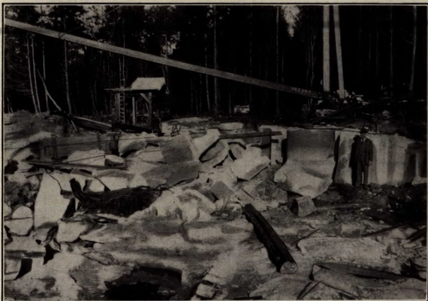
B. The McDonald pulpstone quarry, Newcastle island, B.C., showing 6-foot bed from which circular stones have been cut.
