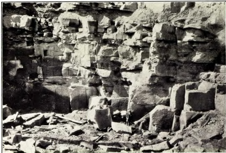
A. Quarry of Miramichi Quarry Company, Quarryville, N.B., showing thick, basal beds from which pulpstones are made.
