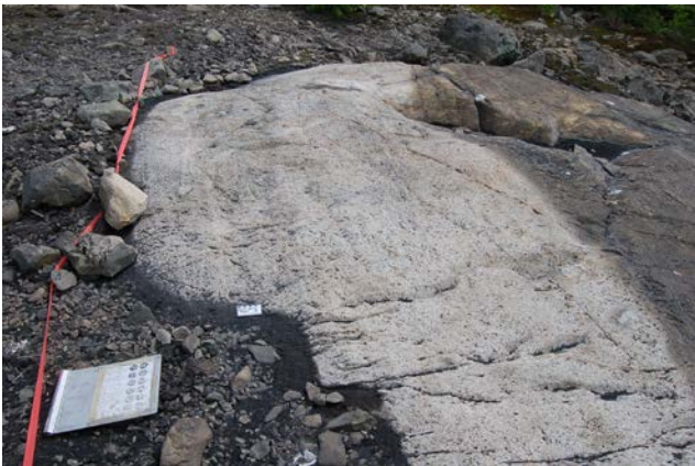
Figure 5.2. b. Example of a part of outcrop cleaned on the left and of a part not cleaned on the right.
