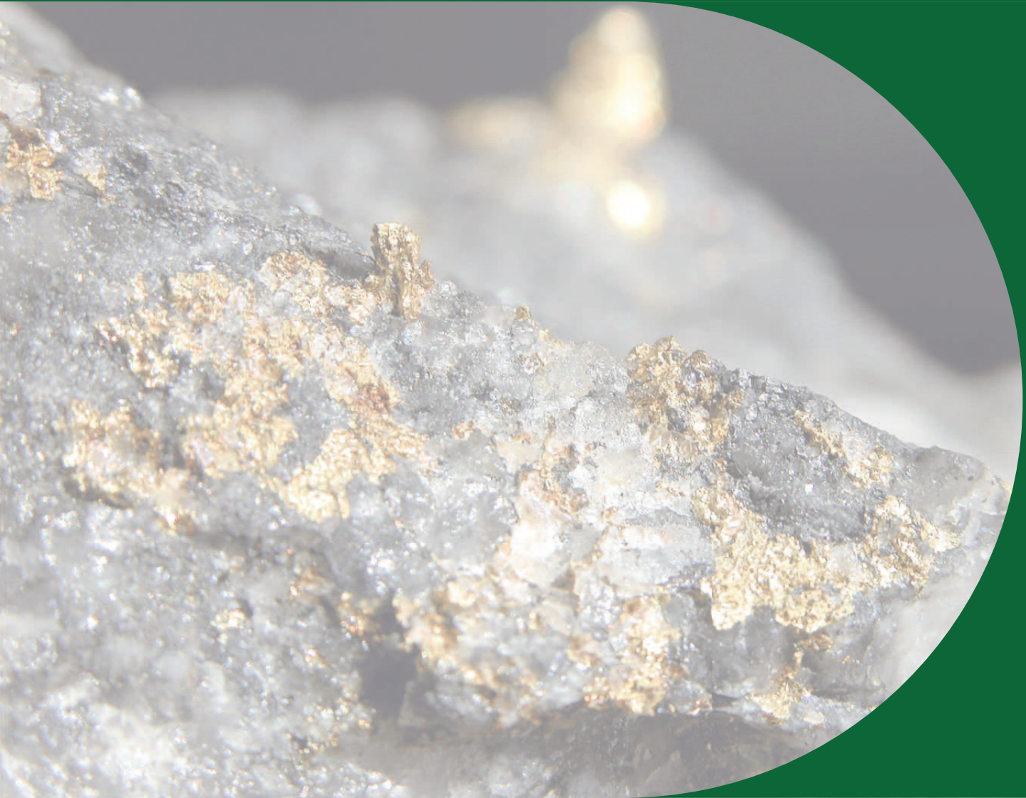
Native gold in a quartz-carbonate vein hosted in strongly iron-carbonatized mafic volcanic rocks from the Lac Fortune area west of Rouyn-Noranda
