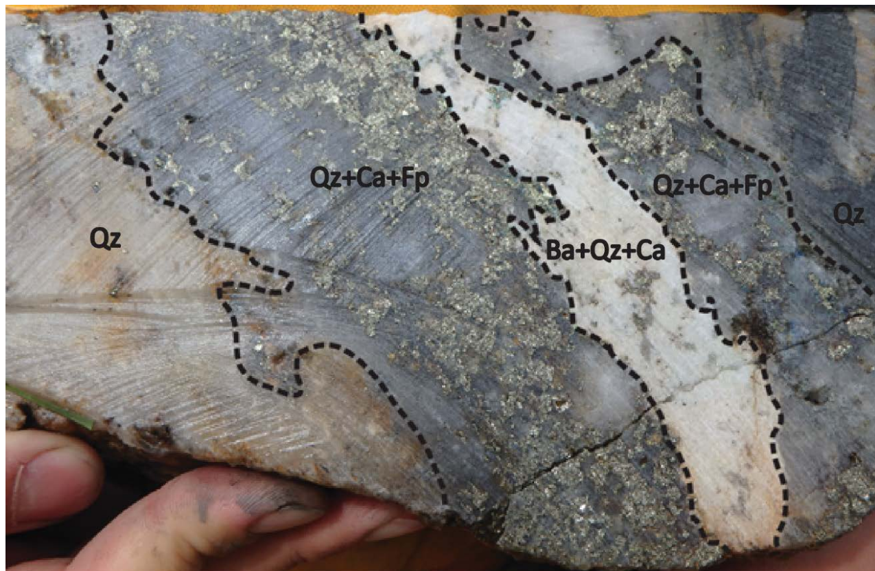
Figure 9.6. Mineralized banded quartz vein showing a well preserved mineralogical zonation with quartz (Qz) at the outer margin, quartz-calcite-feldspath (Qz+Ca+Fp) toward the centre of the vein, and barite-quartz-calcite (Ba+Qz+Ca) directly at the core. Barite is the white mineral.
