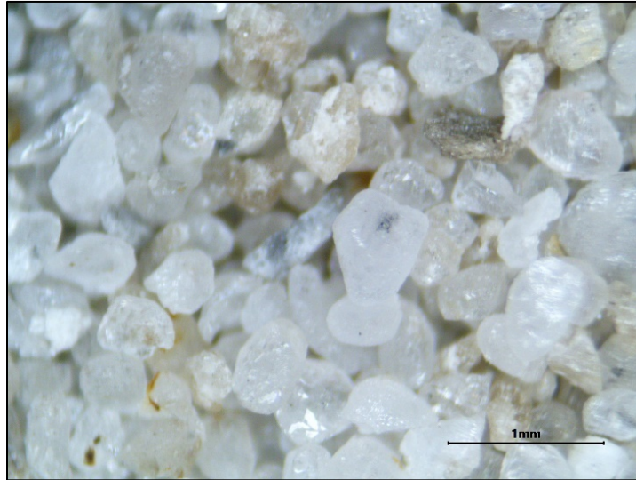
Figure 5: T007168, Cons et al 34150, Mersea, 2, 20-VII. Oriskany Formation. 165m depth. 30x photograph of medium to coarse quartz sand (+minor carbonate) of Oriskany Formation.
