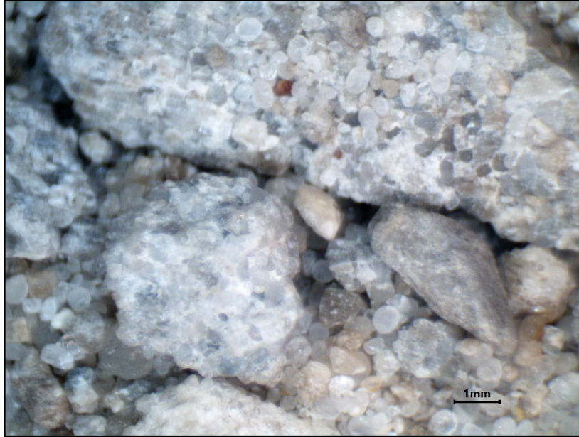
Figure 20: F001709, Ajax Oil and Gas Co. Ltd. No. 12 -R.W. Johnston No. 2, Dover, 3-III. Columbus, 130.45m depth. 10x photograph of loose quartz of Columbus and some aggregated (cemented) quartz grains.
