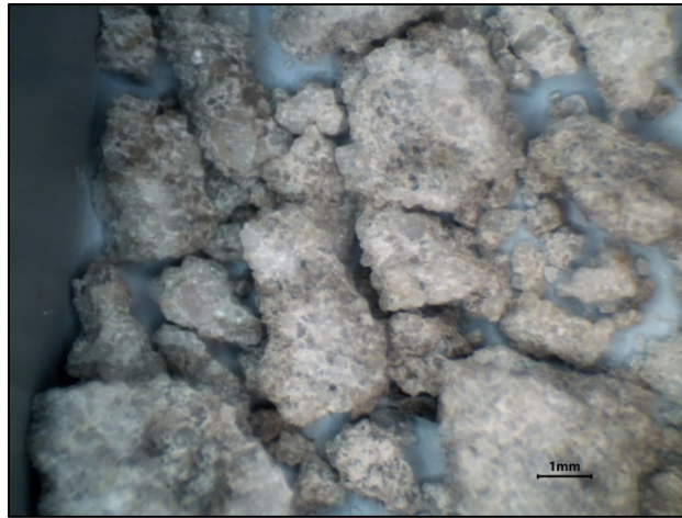
Figure 8: T002803, Consumers' Amoco 13102, Lake Erie offshore, 96-D. Springvale Member. 175.26m depth. 10x photograph of typical Springvale sand; cemented (calcite/dolomite) fine to medium quartz sand with glauconite (green).
