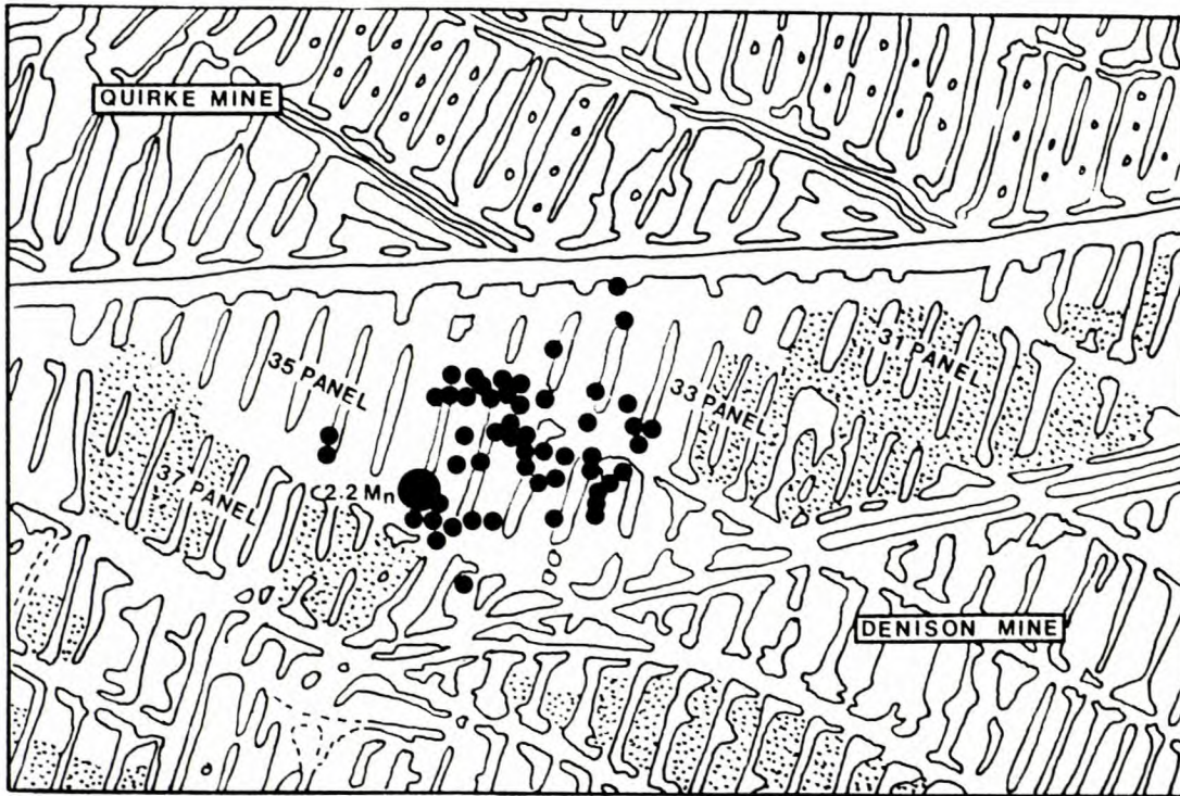
Fig. 6.19 - Location of seismic activity at Denison Mine during May 1987.
