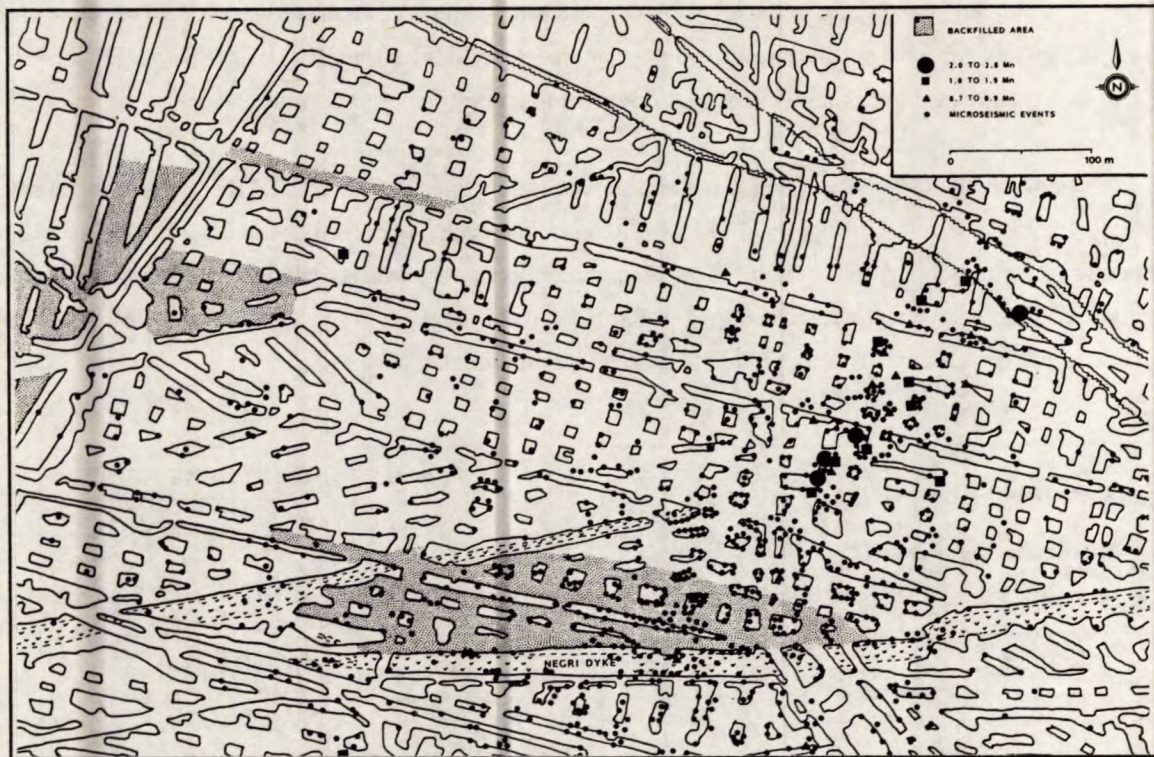
Figure 15 - Plan of the eastern part of Denison Mine showing extent of seismic activity, 1987 to 1989
