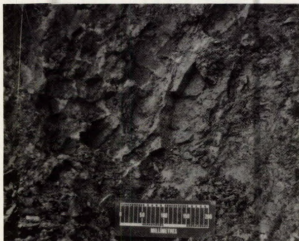
Figure 15 Near surface exposure of weathered Ludlow Shales at steep angle of dip
