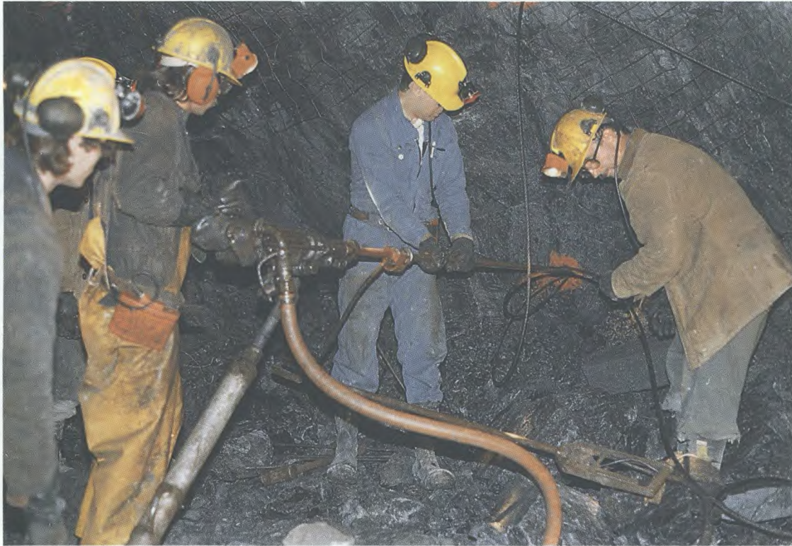
Trial installation of Swellex bolts with steel cables at the Campbell Red Lake Mine.
