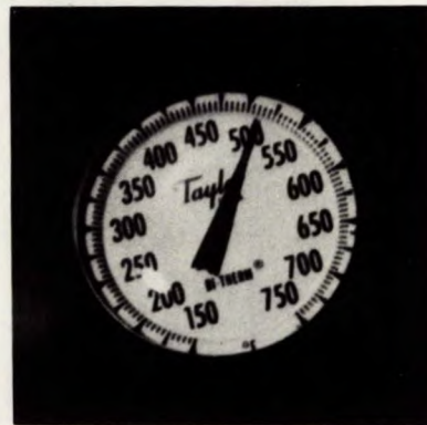
Figure 3.18 Stack temperature measurement
