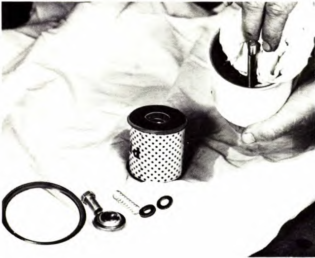
Figure 3.7 Servicing the oil filter
