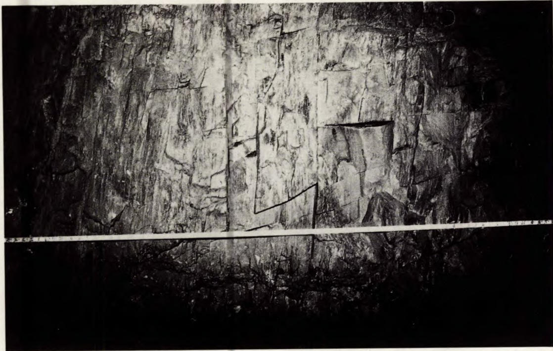
Mine 9, gallery 4: 3.5 fractures/metre (in this location), RQD = 95% 3 major sets, dip = 90°, dip = 20°, dip = 0°
