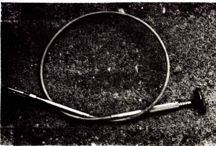
Fig. 15 - Gauge used to measure the diameter of a drill hole. From reference (31).
