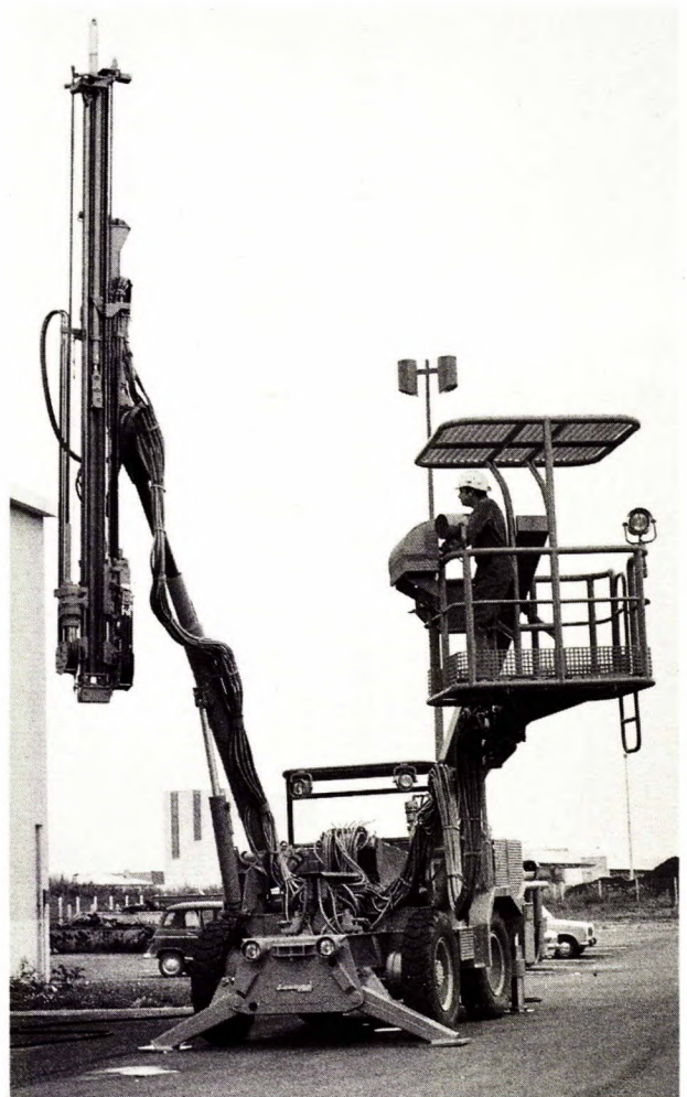
Fig. 75 - Roofbolter for 3.6-m (12-ft) long rockbolts
