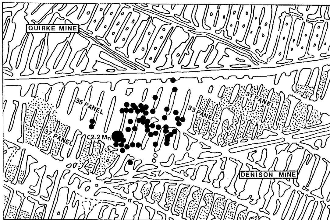
Location of seismic events during May 1986 at Denison Mine. It is of interest, that no seismic activity was recorded in the surrounding backfilled area.
