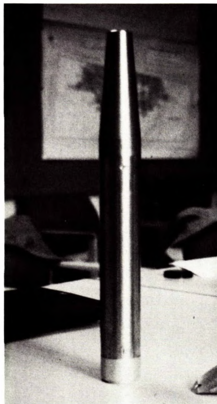
Figure 3. Stainless steel housing for triaxial sensors.
