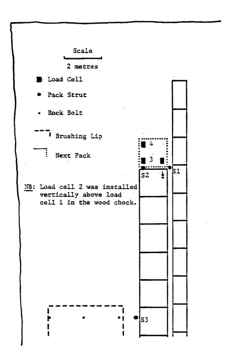
Layout of the 9E Maingate face end and instrumentation at the installation of Site 1
