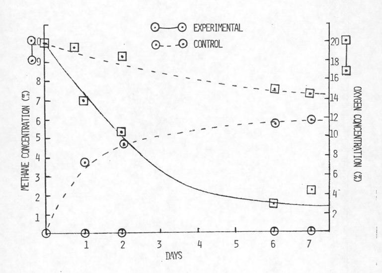
Fig. 3 - Control of methane concentration in a model coal silo. 5 ml cell suspension, 20 ml Bushnell Haas medium, added to 200 g freshly ground coal in a sealed flask.
