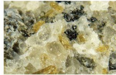
Photomicrograph of carbonate from Oka, Quebec. Mineral assemblage includes rosalia (yellow), calcite (white), pyrochlore (black) and apatite (grey). Field of view is 1 cm. Photo: T. Pearson, GSC.
