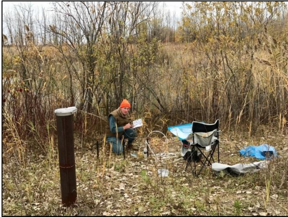
Sampling groundwater piezometers near the old tailings decant pond
