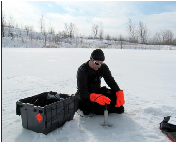
Collecting water quality measurements to a depth of 100 m in Pit #2
