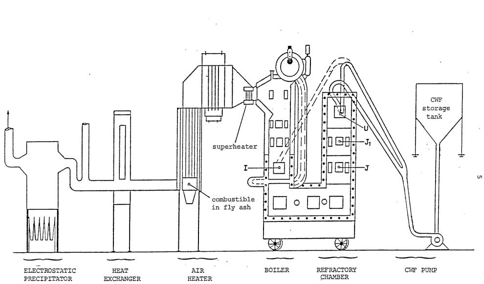
Fig. 1 - Schematic of CCRL pilot-scale boiler with CWF handling system
