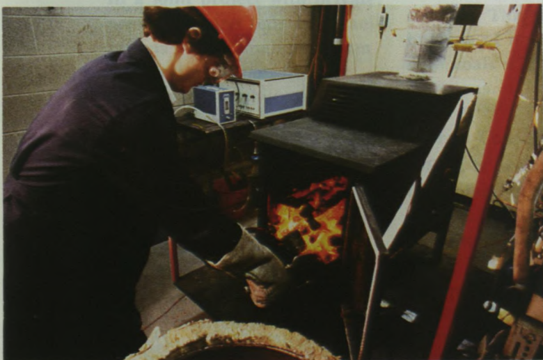
Combustion efficiencies and other combustion properties of biomass fuels are tested in this domestic wood stove.
