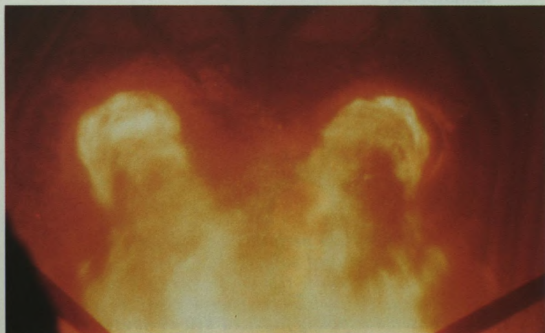
A coal-water fuel flame in a utility boiler. This fuel offers advantages relative to both pulverized coal and oil.
