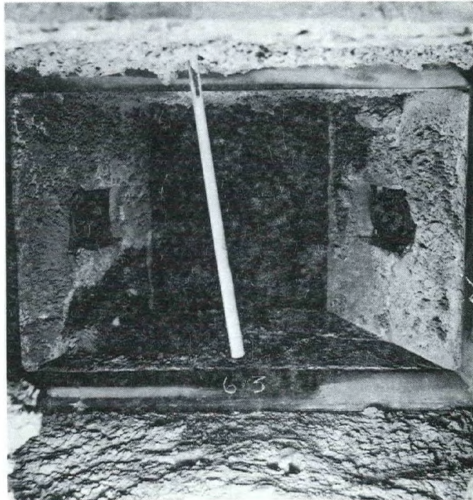
FIGURE 1a Furnace bottom at end of test. Burners and furnace throat are clear of sinter. Air cooled deposition probe in foreground projects from east wall. Remains of refractory deposition probe may be seen across from it on west wall.
