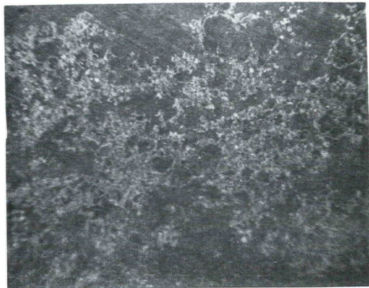
Figure 1g Photomicrograph, x 10, of a thin section of sinter which was found attached to the refractory near the burners. The sinter is weak and porous.
