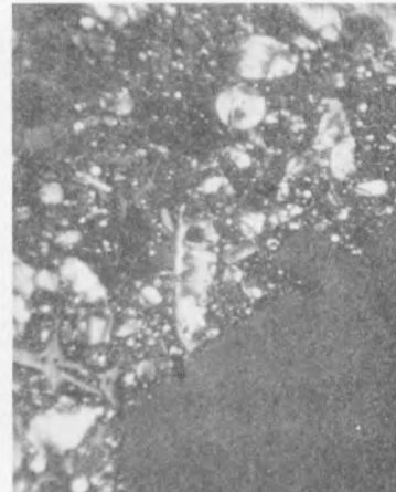
Figure 3. Spheroidal structure in the hydrogenated lignite.
