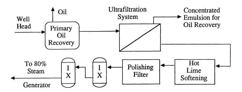
Figure 2 Flow Schematic for Membrane Test Equipment
