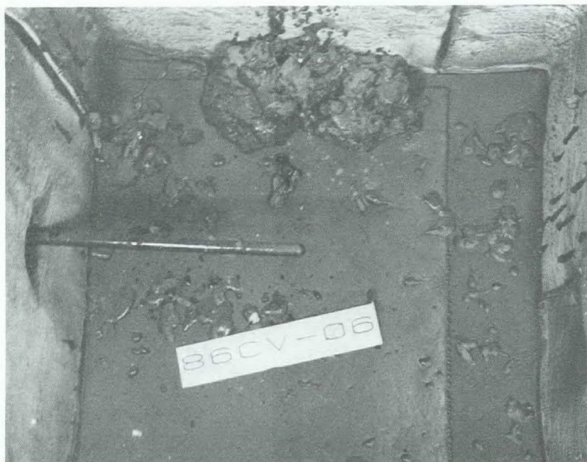
Fig. 7 - Deposits in furnace bottom
