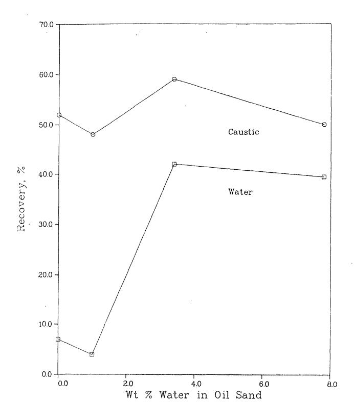
Figure 7: Effect of connate water saturation added during reconstitution on recovery.
