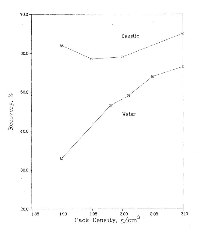
Figure 6: Influence of oil sand compaction density on recovery.
