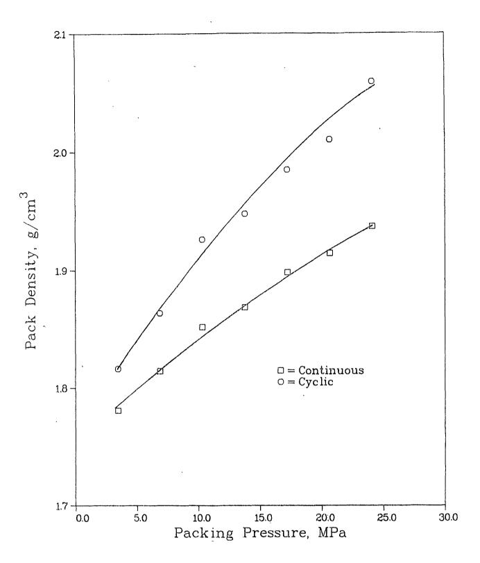
Figure 2: Influence of packing procedure on resultant oil sand density.
