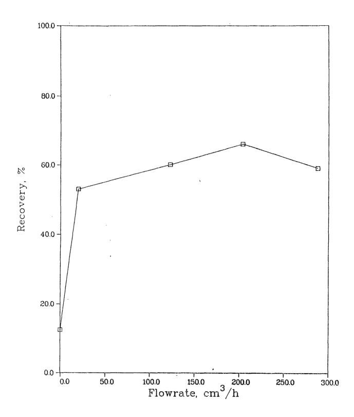
Figure 5: Influence of flowrate of caustic on displacement efficiency.
