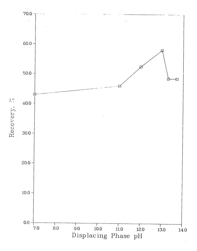
Figure 9: Effect of displacing phase pH on recovery.
