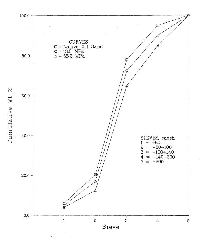
Figure 3: Sand size distribution related to compaction pressure.
