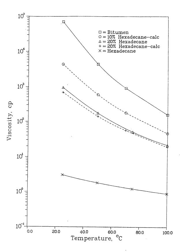
Figure 1: Comparison of calculated and measured mixed liquid viscosities.
