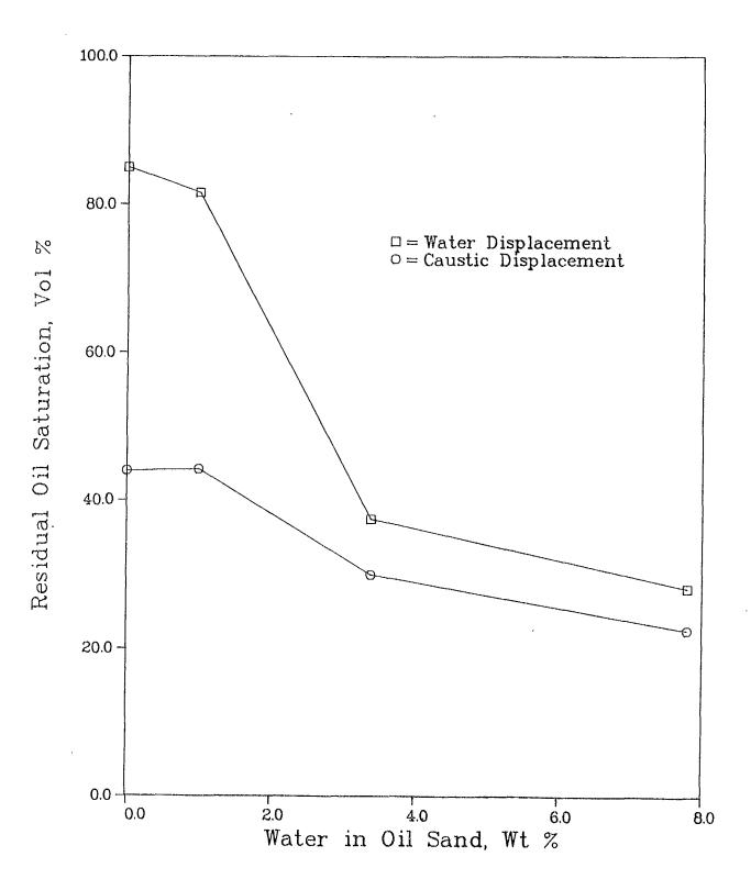
Figure 8: Effect of connate water saturation added during reconstitution on residual oil saturation.
