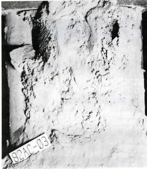
FIGURE 13. Superheater blockage due to chloride addition to dolomite and coal ( \text{Ca} + \text{Mg}:\text{S} = 4.5 ).
