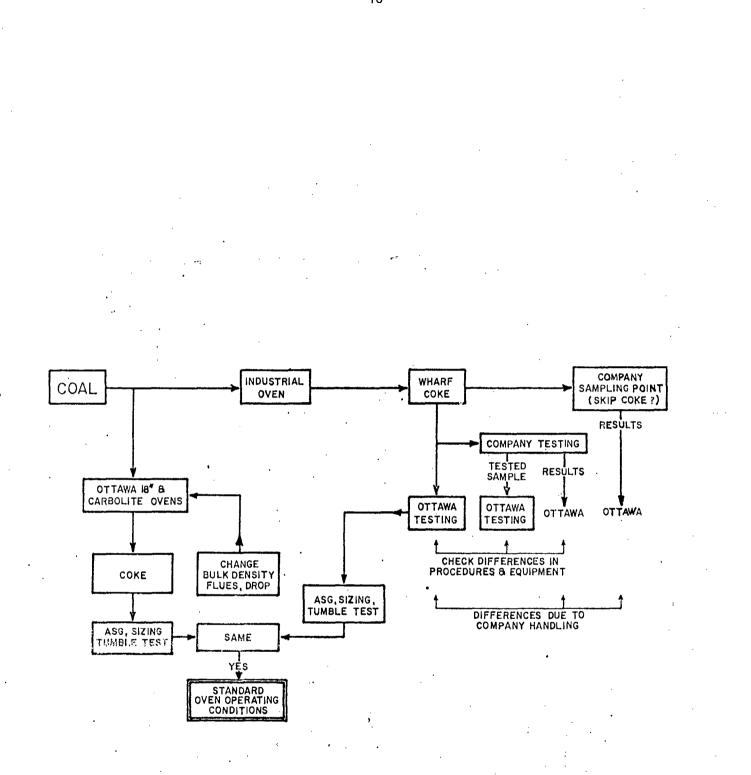
Fig. 1 - Sampling and analysis routine for commercial and technical oven comparisons.
