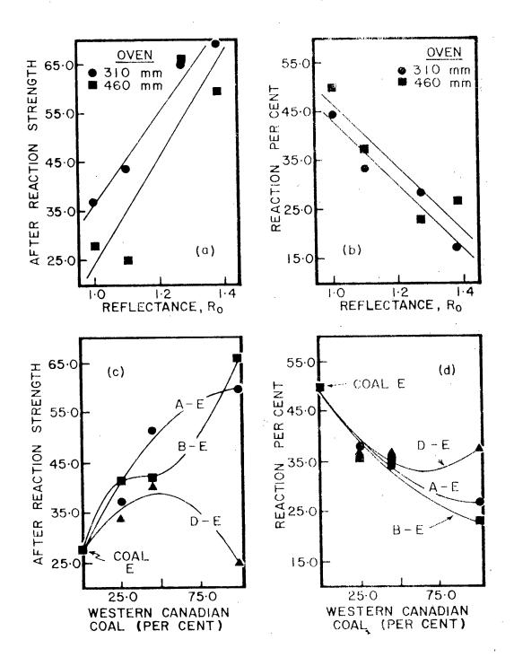
Fig. 5 - The after reaction characteristics of coke produced from binary blends of Canadian coals.
