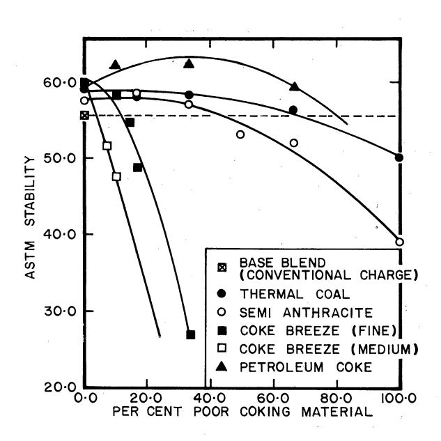
Fig. 9 - The addition of non-coking materials to partially briquetted coal blends.
