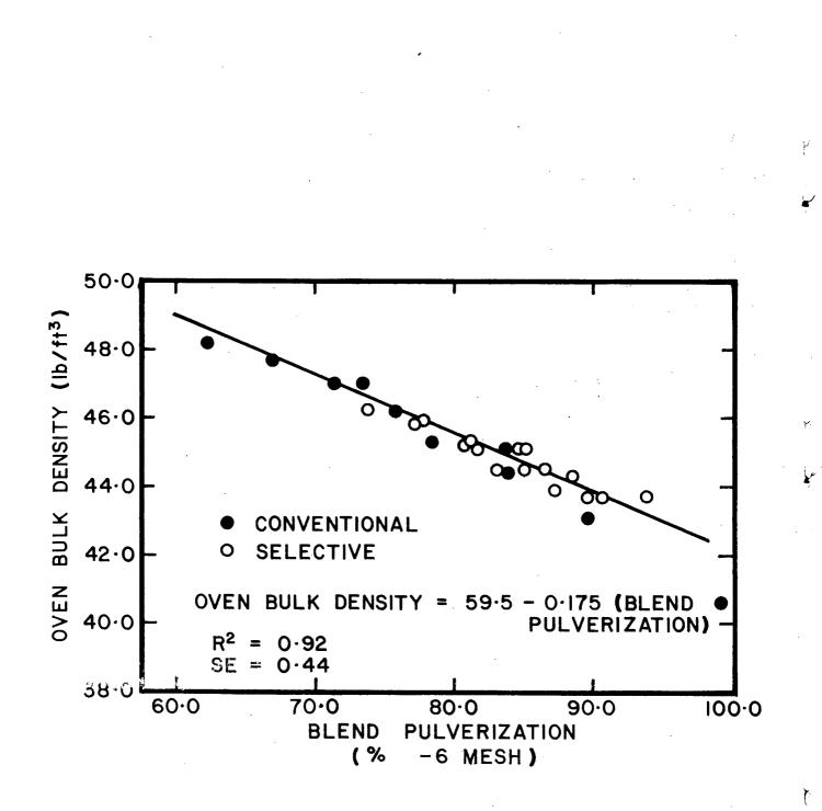
Fig. 7 - The effect of selective pulverization on coke quality
