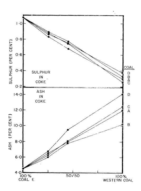
Fig. 6. - The sulphur and ash content of cokes produced from binary blends of Canadian coals.
