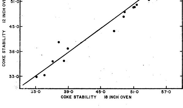
Fig. 3 - The coke-stability correlation between the two Ottawa ovens
