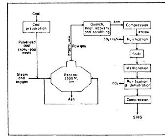
There are 16 commercial plants operating to produce a synthesis gas for ammonia production. The process is under consideration for current installation.
