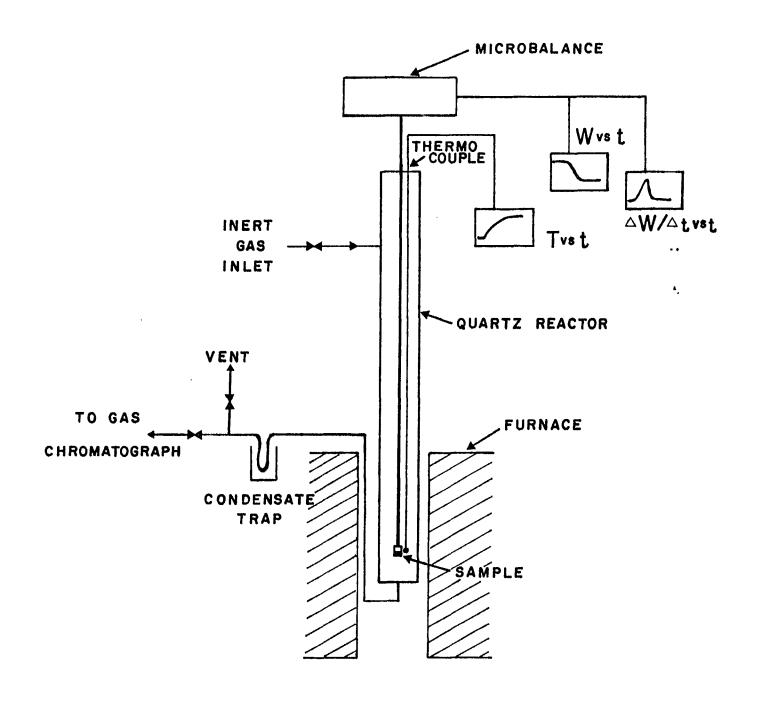
SCHEMATIC DIAGRAM OF THE MICROBALANCE REACTOR
