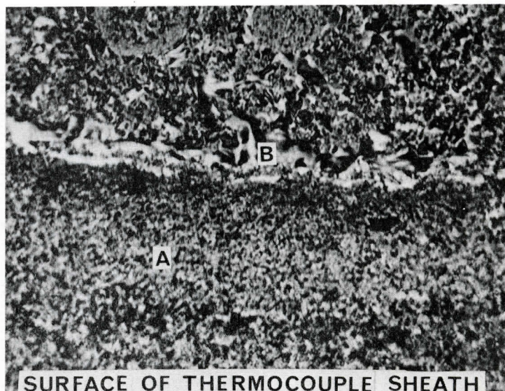
FIGURE 4 - Coke Deposited on the surface of the Thermocouple Sheath in the Reactor During Thermal Hydrocracking of Athabasca Bitumen; 450°C, 10.44 MPa (x 600) A - grain-mosaic structure B - flow-type structure
