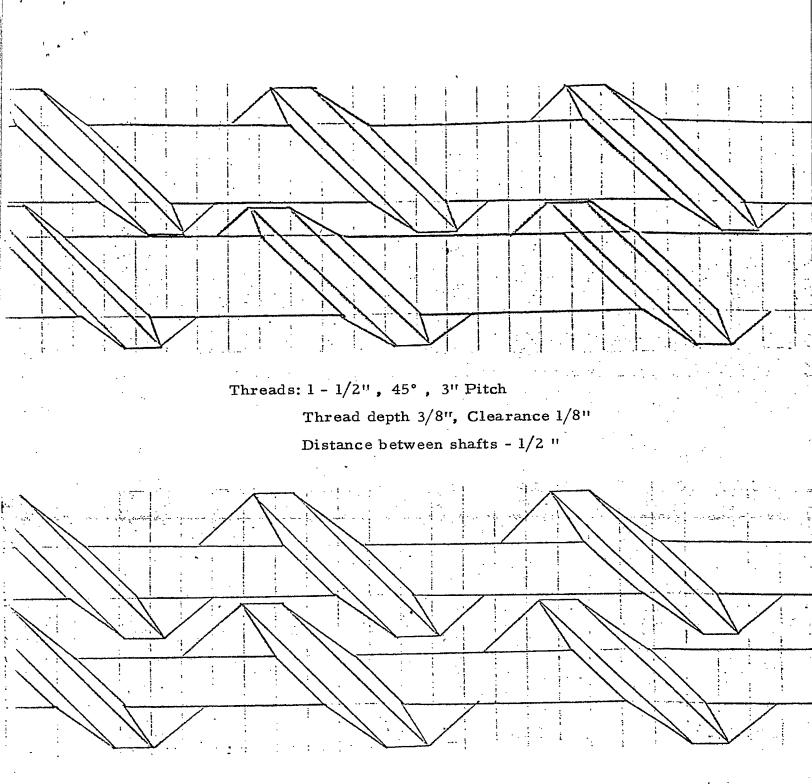
Threads : 1 - 1/2", 45°, 3" Pitch Thread depth 1/2 " clearance 1/8" Distance between shafts - 5/8"
