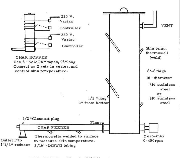
CHAR FEEDER - 4'long by 7/8" diameter screw, threads extend into char hopper. -Heat with one 8'long by 1-3/4"SAMOX tape - Fabricate from 316 or 310 SS, and use
