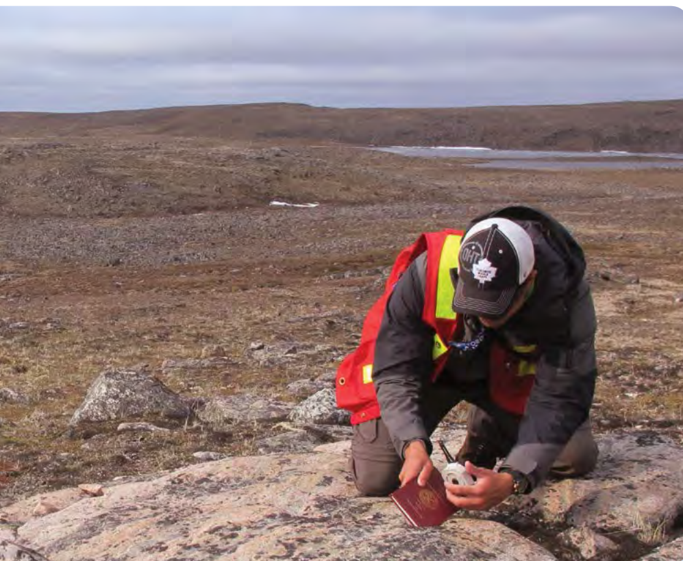
A field assistant takes structural measurements on an outcrop after collecting a sample of granitic gneiss west of Lorillard River, Nunavut.
