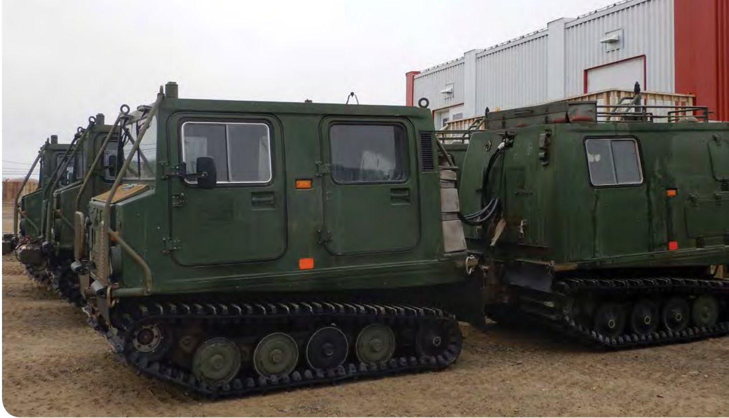
DND Bandvagn 206 (Bv 206) amphibious vehicles at the PCSP facility in Resolute are used for CAFATC training activities.
