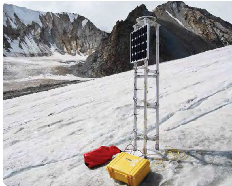
A University of British Columbia/Simon Fraser University solar-powered global positioning system (GPS) tower stands on an unnamed glacier in the St. Elias Mountains, Yukon.
