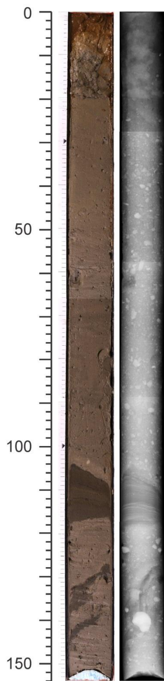
Figure 3.28b. Photography and X-radiography compilation for trigger weight core 2013029-057.
