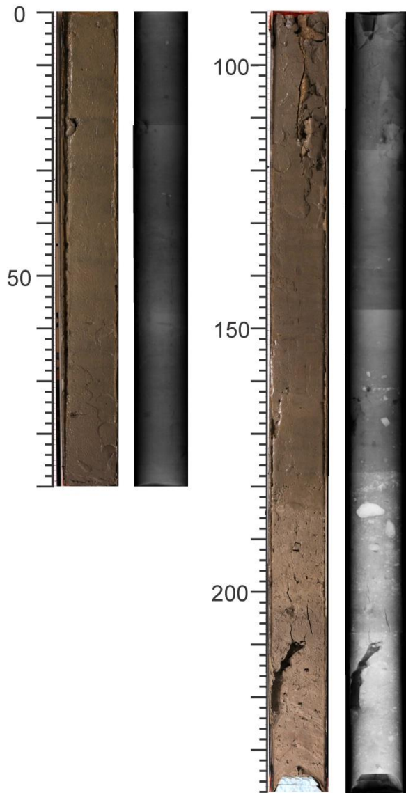
Figure 3.56b. Photography and X-radiography compilation for trigger weight core 2013029-077.
