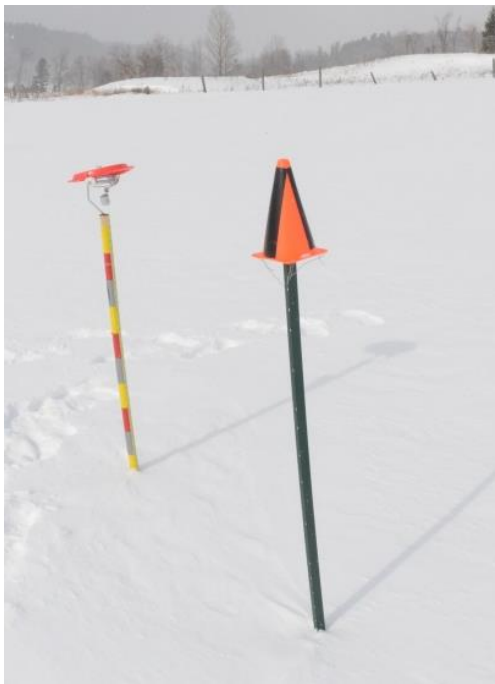
Figure 8. In-situ GCP targets: a) Flat, b) Disk on Pole, c) Disk and Cone on Pole, snow free d) Disk and cone on pole after 15cm snowfall.
