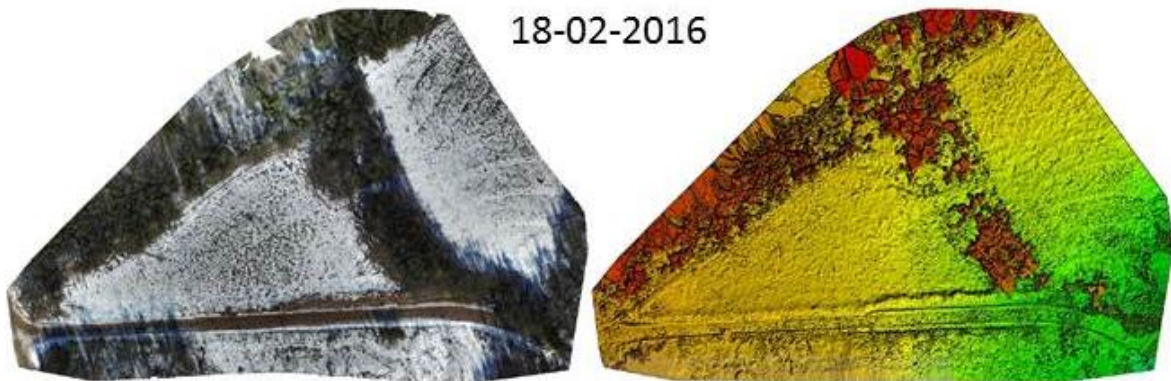
Figure 25. Acadia A orthoimages (left) and DSMs (right).
